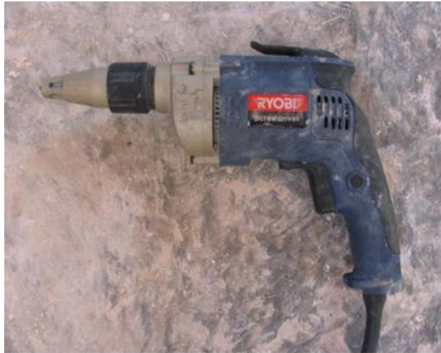
A screw gun adjusted to countersink screws properly is a must.
